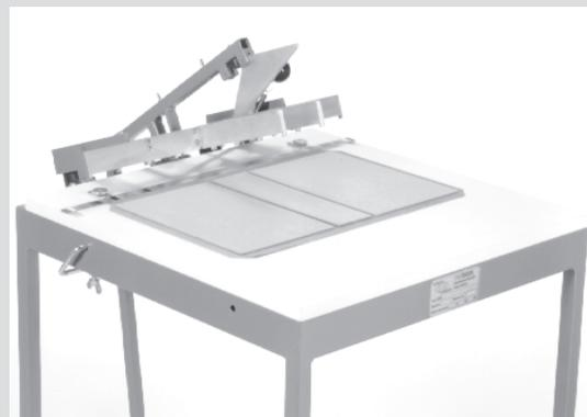
After positioning the cover material, the guide angles are lowered by foot-treadle. At that time, the spine hollow has already been put between the joint bars and is fixed by them. Now the blade presses down the spine hollow. At the same time, the two cardboards are placed into the guide angles (left and
